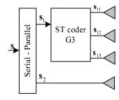
Fig. 2. Architecture of the HMTS G3+1 transmitter
